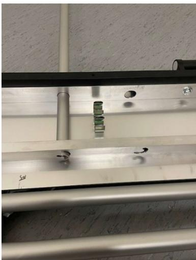
4. Now place the device back on a flat surface and position the supplied adjusting rings on the two length stop tubes at the desired depth using the measuring scale. see illustration
