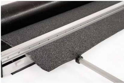
4. Pull the sliding carriage towards you and cut the bitumen sheet in one go if possible.
