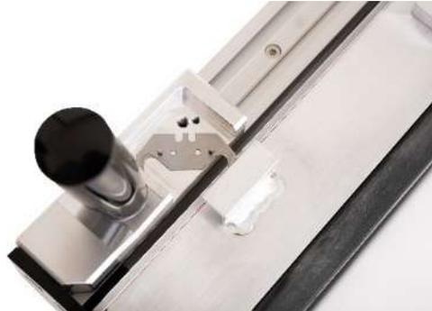
6. Move the sliding carriage into the parking position, where it is held by the built-in holding magnet in the area of the protective strip to avoid cuts.
