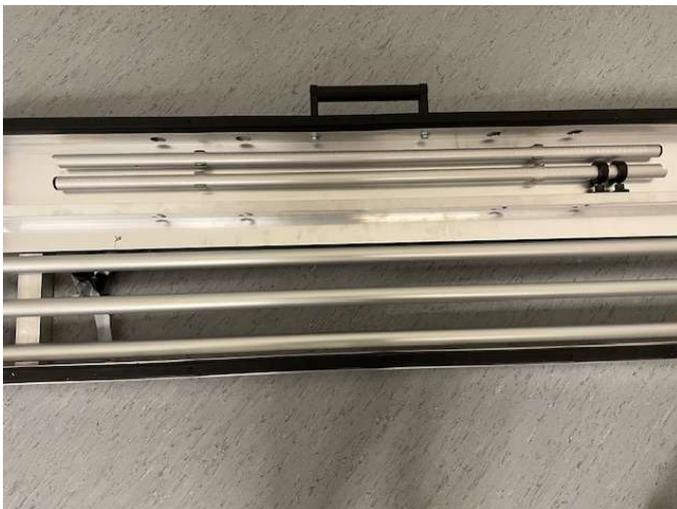
3. Depending on the width of the bitumen sheet, push the length stop tubes into one of the 4 openings all the way to the back and fix them with a clockwise rotation (bayonet).
